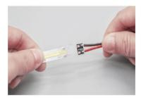
Insert one end of led strip and wire connector into both ends of the connection terminal respectively to ensure that the metal clip is on the same side as the metal solder pad of led strip.
